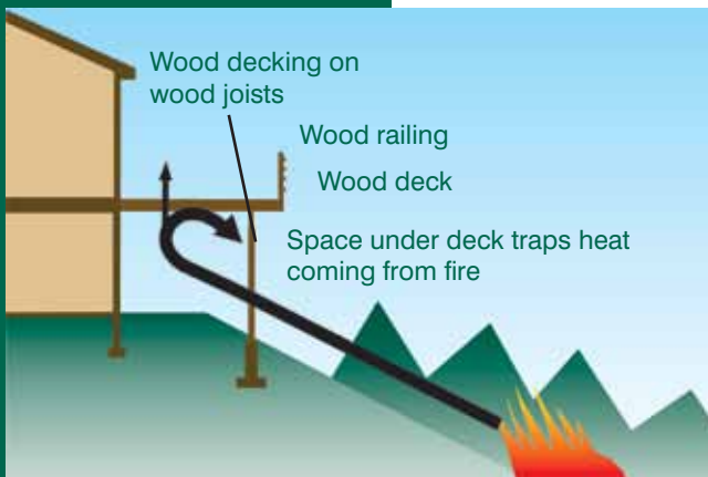
Figure 4-10: Conventional deck in a fire
