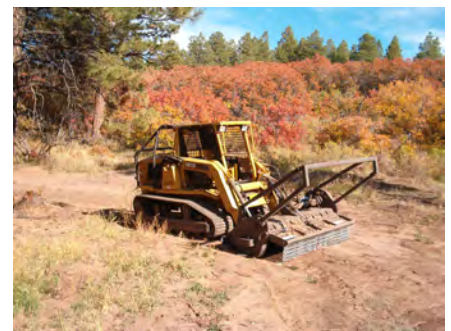
Figure 4. Mechanical treatment using a timberaxe.
