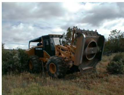
Figure 3. Mechanical treatment using a Hydroaxe®.
